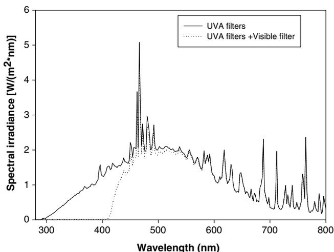
Fig. 1. Irradiation spectra of the xenon arc lamp equipped with UVA and UVA/visible filters used with the Atlas Suntest CPS+. Solid line: Irradiation spectrum of the xenon lamp equipped with the UVA/visible filter (315–800 nm). Dotted line: Irradiation spectrum of the xenon lamp equipped with the visible filter (400–800 nm).
