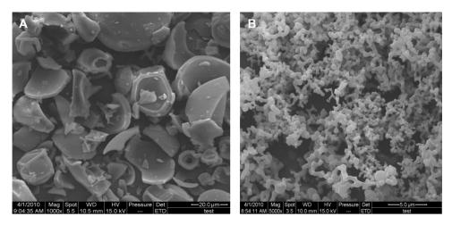
Figure I Scanning electron microscopy result of (A) unprocessed GA and (B) GA nanoparticles. Abbreviation: GA, glycyrrhizic acid.
