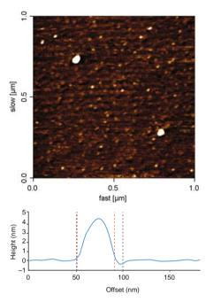
Fig. 1. AFM image of nanoparticles showed distinct spherical particles in size ranging between 50 and 100 nm.
