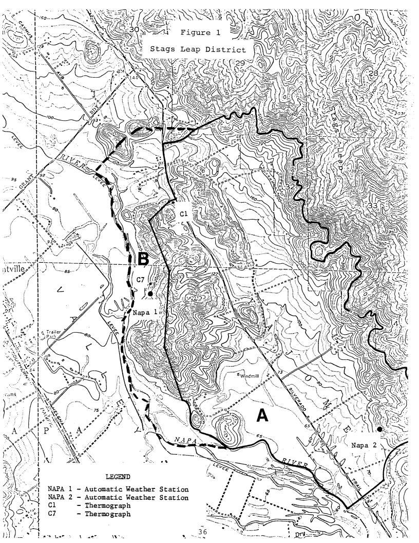
of approximately 180 feet above sea level. Each station was programmed and installed with instruments to measure temperature and humidity at the two meter height and wind speed and direction at a height of three meters. The observations were averaged over half-hour intervals and stored on magnetic tape. The tapes were then read into a microcomputer for processing. Data contained in this report were gathered from the stations between September 26 and November 9, 1985.
